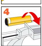
4. Place the cartridge into the application gun ready for use
