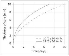
Diagram 1: Curing speed Sikaflex®-271
