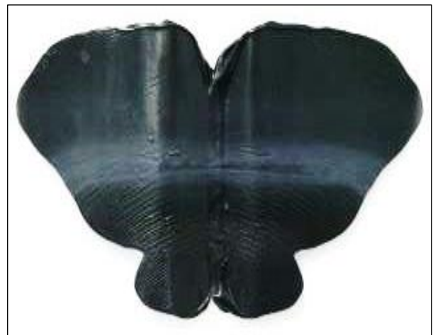
FIGURE 12 Unfold the foil - Negative test = inadequate mixing
