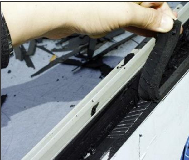
FIGURE 19 Good adhesion, deglazing test positive
