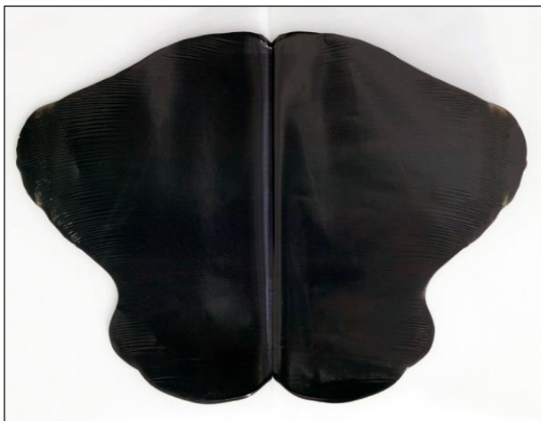
FIGURE 11 Unfold the foil - Positive test = ideal mixing
