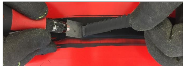
FIGURE 18 Peel adhesion test on enameled glass: cutting the bead while pulling
