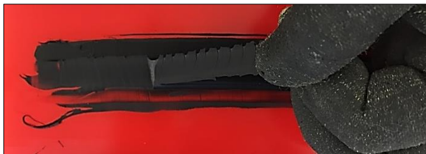
FIGURE 17 Peel adhesion test: pulling the bead apart, 100 % cohesive failure occurring
