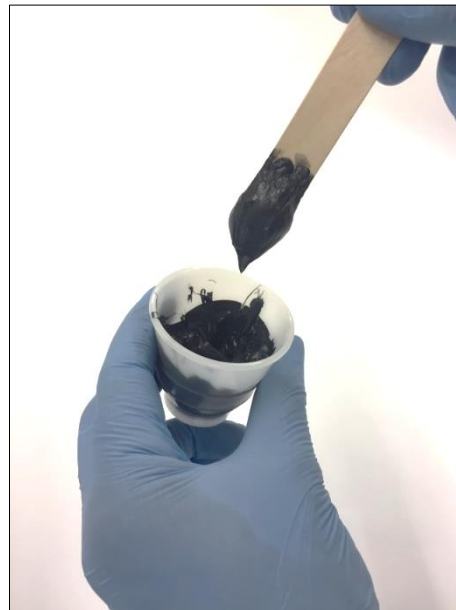
FIGURE 15 Material shows rubber-like behavior: → snap time reached
