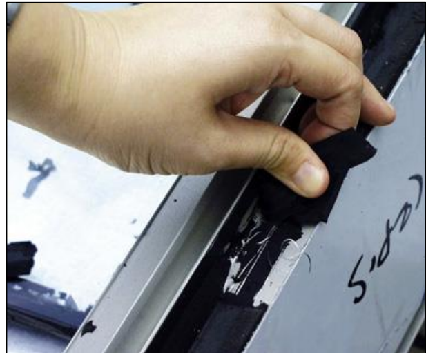
FIGURE 20 Adhesive failure, deglazing test negative
