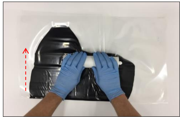
FIGURE 10 Press the bead only in direction perpendicular to fold
