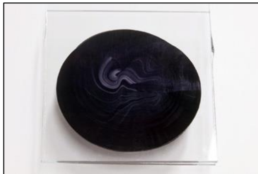
FIGURE 8 Negative test = inadequate mixing
