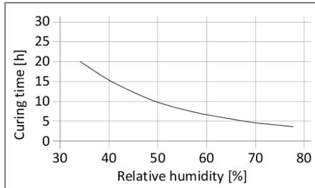
Diagram 1: Curing time for 500 µm film
