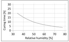
Diagram 1: Curing time for 500 μm film
