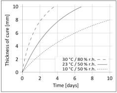
Diagram 1: curing speed Sikaflex®-252
