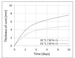
Diagram 1: Curing speed Sikaflex®-522
