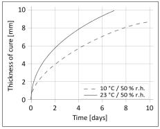
Diagram 1: Curing speed Sikaflex®-223
