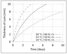
Diagram 1: curing speed Sikaflex®-252
