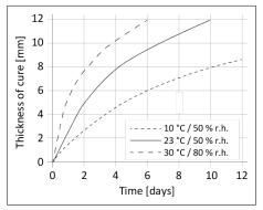
Diagram 1: Curing speed Sikaflex®-250 PC
