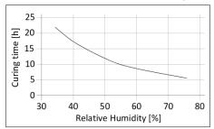
Diagram 1: Curing time for 500  $\mu m$  film
