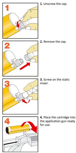
When the work is interrupted, the static mixer nozzle can remain on the cartridge after the gun pressure has been released. If the resin has hardened in the nozzle when work is resumed, a new nozzle must be attached.
