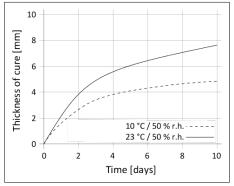
Diagram 1: Curing speed Sikaflex®-522
