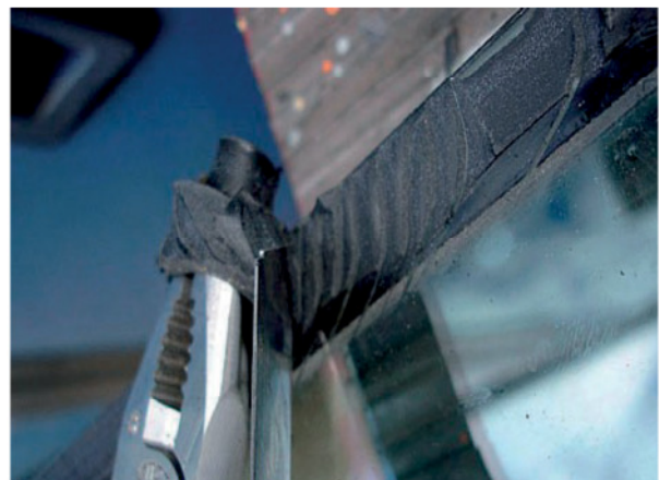
Good adhesion on unprimed ceramic
