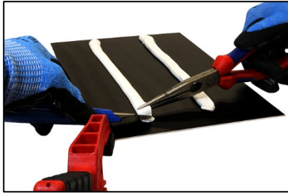
Figure 14 After complete curing, separate the first 2 – 3 cm of the bead
