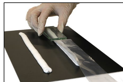
Figure 13 Press the bead to half the height
