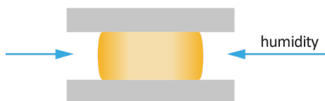
Figure 1 Humidity curing principle
