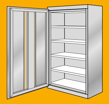
Stiffener bonding: **SikaPower®-880** can also be applied before the painting process. For pre-coated surfaces: Sikaflex®-552 AT or for faster assemblies, Sikaflex®-953 can be used.
