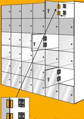
Stainless steel hinges bonded on steel: SikaFast<sup>®</sup>-555 LO5.
