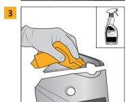
Clean entire work area using Sika® Cleaner G+P. making sure the surface is completely dry and no moisture remains
