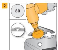
Grind a V-groove (1 cm approx.) into the side edges, use 80 grit sandpaper
