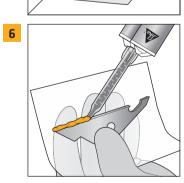
Position the broken part on the Sika Contouring Film and apply Plastic Adhesive Superfast on the breaking
