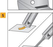
Before attaching mixer, extrude some material until both parts A and B flow evenly
