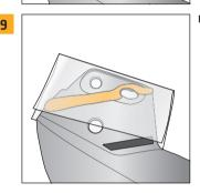
■ Bend the film and compress adhesive and wait for adhesive to be cured according to product label
