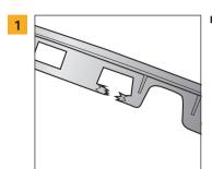
■ Damage: a broken eyelet
