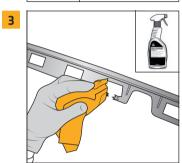
Clean entire work area using Sika® Cleaner G+P, making sure the surface is completely dry and no moisture remains
