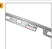
Compress tape and adhesive and wait for adhesive to be cured<sup>1)</sup> according to product label
