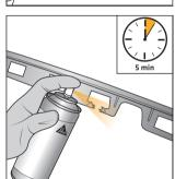
■ Spray a thin coat of Plastic Primer on both sides, flash-off for 5 min<sup>1)</sup>
