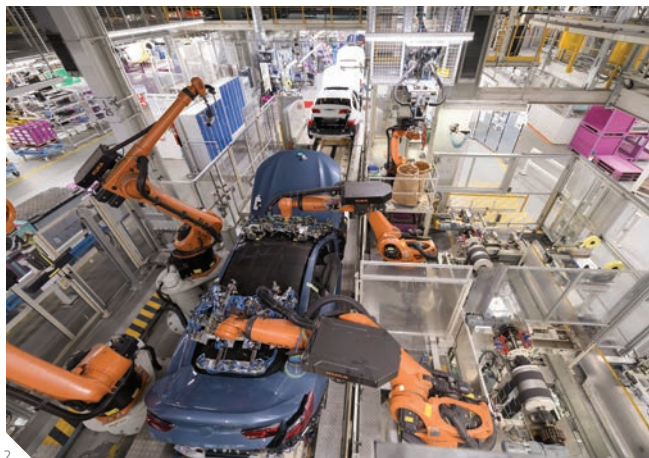
1 Automated application of Sikaflex® 2 Automated bonding of windshield
