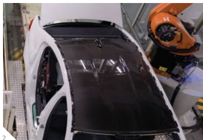
1 Crash resistant bonding of mixed material 2 CFRP roof bonding
