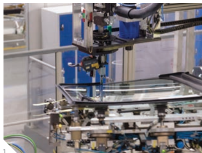
1 Automated application of Sikaflex® 2 Automated bonding of windshield
