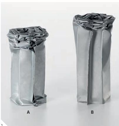
1 **IMPACT TEST RESULTS:** (A) Spot welded
