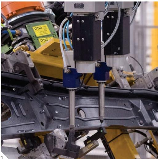
1 SikaPower® MBX - Central tunnel bonding (CFRP - steel)
