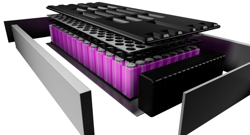
Potting of cylindrical cells in modules
