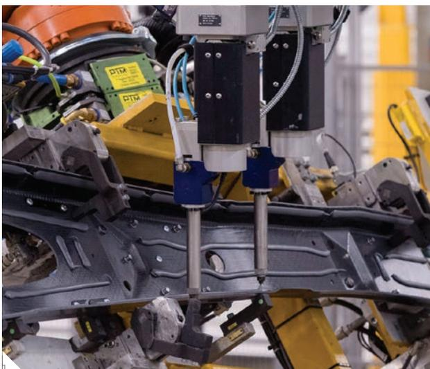
1 Central tunnel bonding (CFRP - steel)
