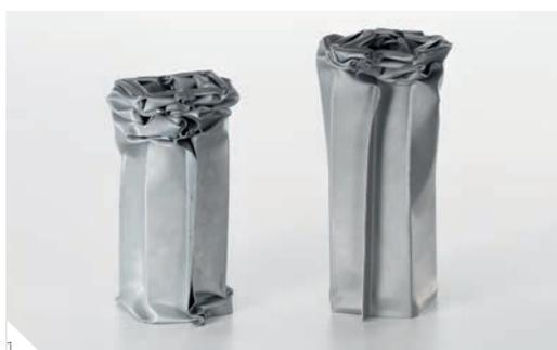
1 Crash beams without (left) and with SikaPower® (right)
