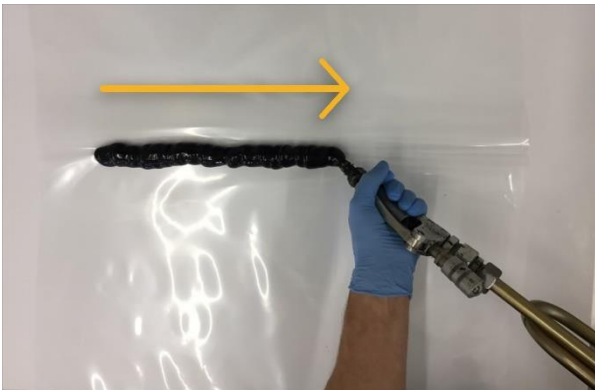
Figure 4: Apply the bead in the fold direction
