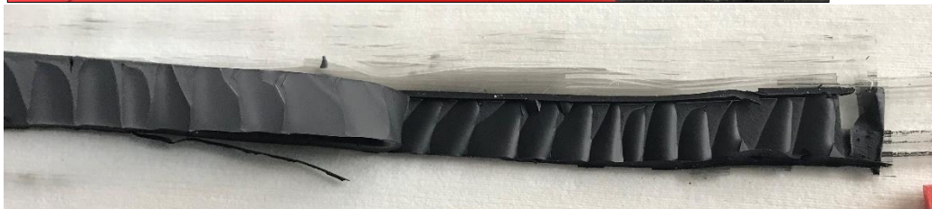
Figure 19: Peel adhesion test: pulling the bead apart; result: 100 % cohesive failure
