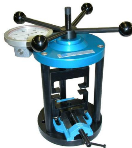
“Ban VEC” manual test bench with analog measurement (sold by GINGER CEBTP);
