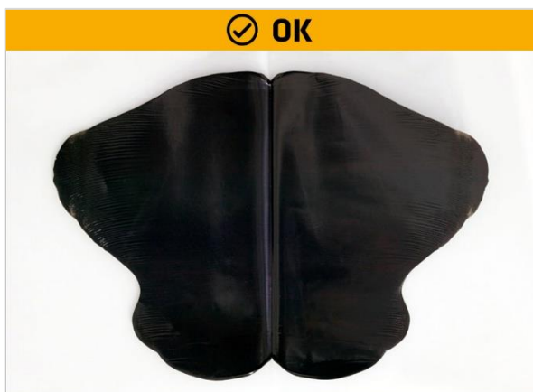
Figure 6: Unfold the foil - Positive test = ideal mixing
