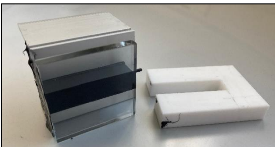
Figure 25: Remove the white, U-shaped Teflon-spacer after the relevant curing times (see above)
