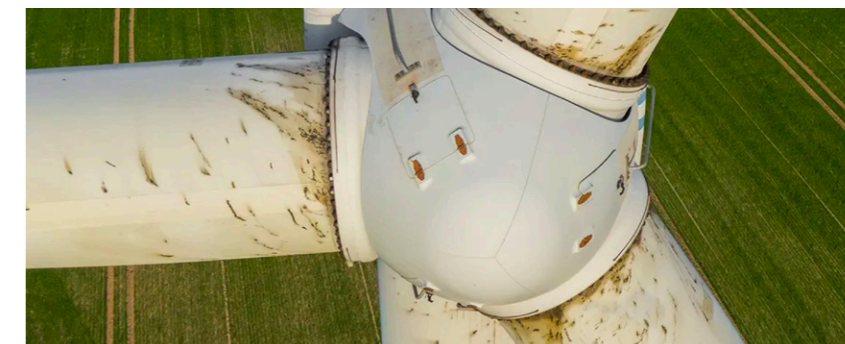
Oil spills from blade pitches.
