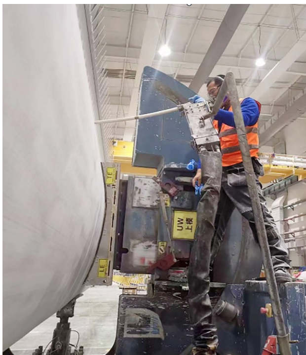
Balancing of a wind turbine blade after production.
