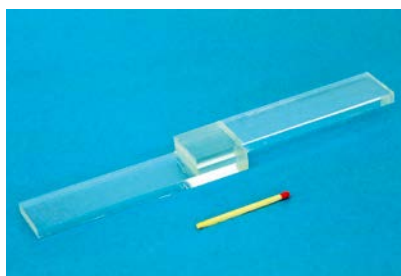
Fig. 3 Test sample. Lap shear test with PMMA substrate bonded with different adhesives. One sample has been screwed
