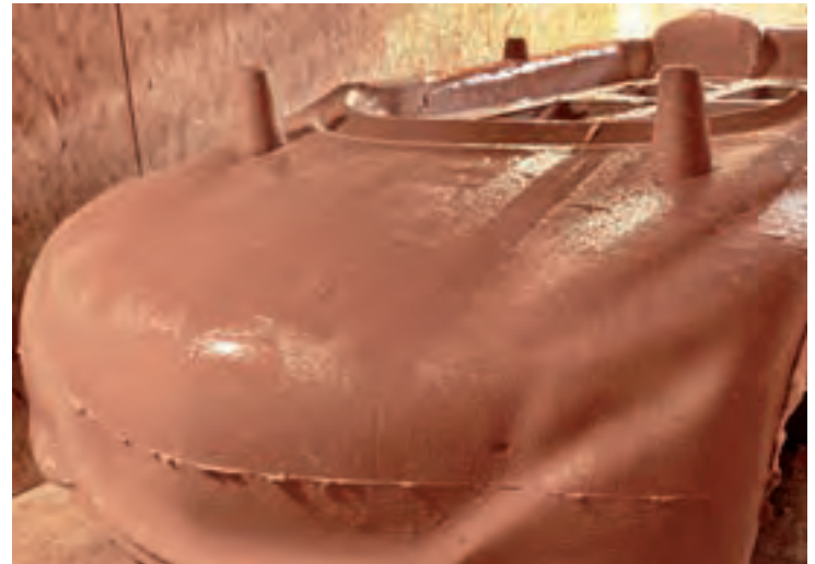
Also huge models in scale 1:1 can be casted out of Biresin® M67 in one shot
