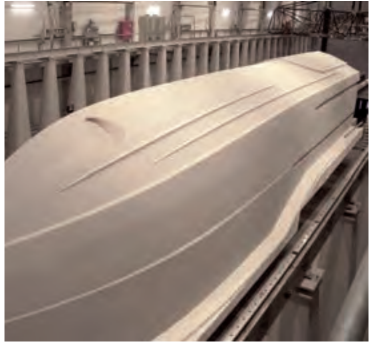
43 m long boat hull made of SikaBiresin® SC175 with a perfectly smooth and seamless surface
