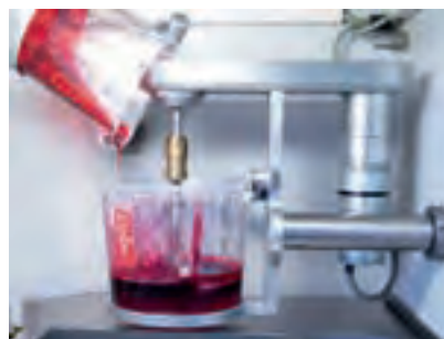
Vacuum casting process provides parts with best visual appearance and highest mechanical properties
