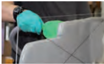
SikaBiresin® SC175 thixotropy enables vertical application in single layer and without sagging
