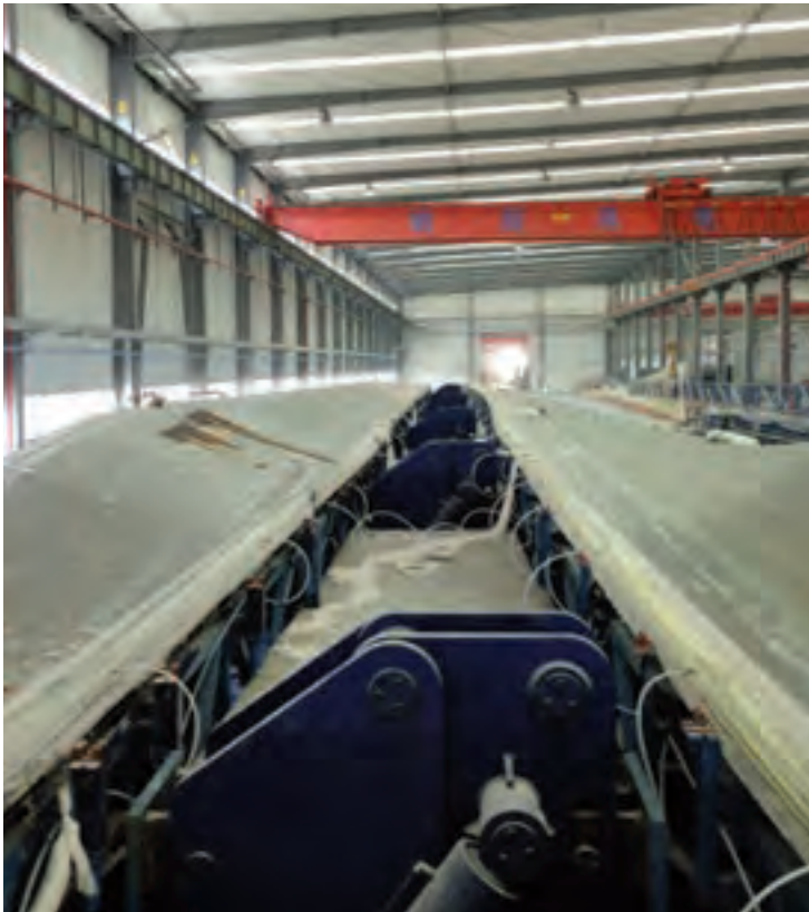
Vacuuminfusion of a wind blade with SikaBiresin® CR131
