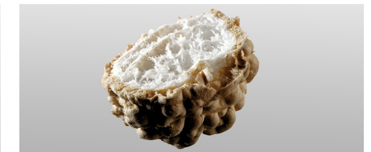
Palusol® after reaction with fire: heat-insulating and pressure-resistant foam
