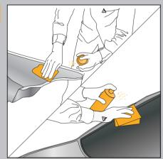
Clean target bonding areas with a suitable residue-free solvent
