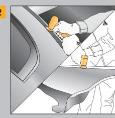
■ Grind bonding areas on both car body and new panel to bare metal
