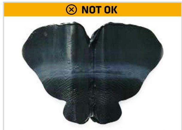
Figure 8: Unfold the foil - Negative test = inadequate mixing
