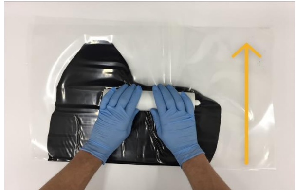
Figure 6: Press the bead only in direction perpendicular to fold
