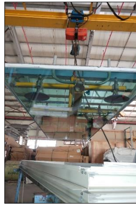
Figure 36: Glass pane completely removed from frame.
