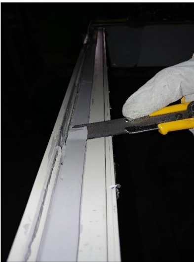
Figure 37: Testing joint adhesion along the whole frame – Good adhesion.
