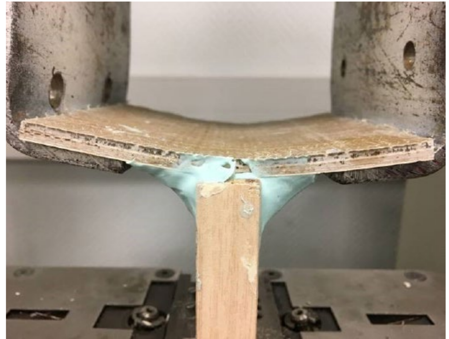
Bulkhead-Composite test sample. Thanks to its unique elastic distorsion Adekit A236 absord the stress applied on the structure: THE COMPOSITE IS NOT DAMAGED.
