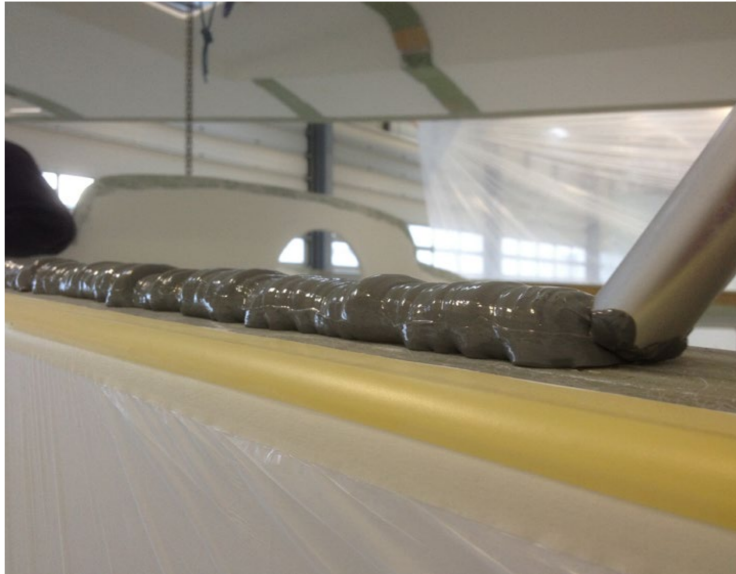
Adekit A236 dispensing on hull. Up to 5 kg/minute with standard dosing equipment for time saving in production.
