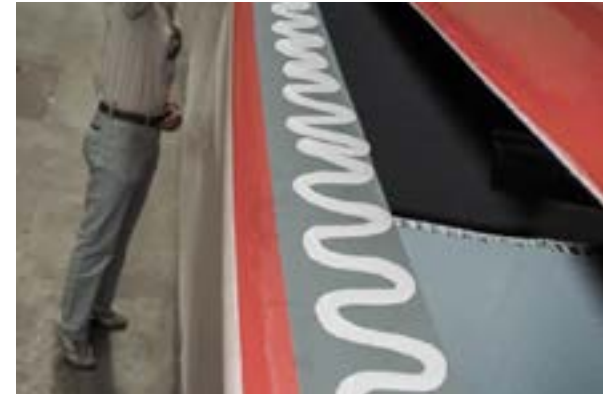
Sikaflex®-292i is applied in a thick layer on the bonding surface
