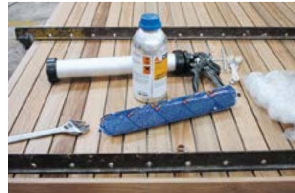
Deck clamped for curing
