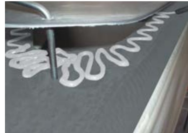
A locating pin helps to accurately align the adhesive bead
