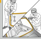
■ Apply a triangular bead of adhesive either to the glass or the aperture
