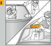
■ Cut out damaged windshield using Sika SmartCut, electrical knife, cutting wire, cold knife etc.
