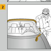
Cover the aperture with masking tape
