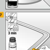
■ Prime the bonding surface of the glass using Sika® Primer-207
