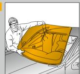
Remove damaged windshield
