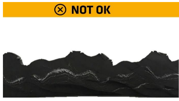
Figure 16: Severe white stripe in material, inhomogeneous mixing
