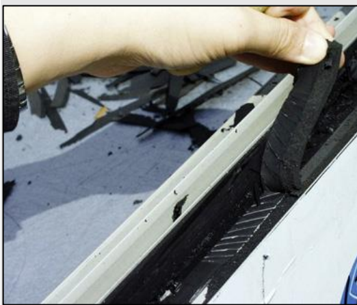
Figure 26: Good adhesion, deglazing test positive
