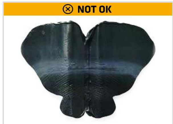
Figure 12: Unfold the foil - Negative test = inadequate
