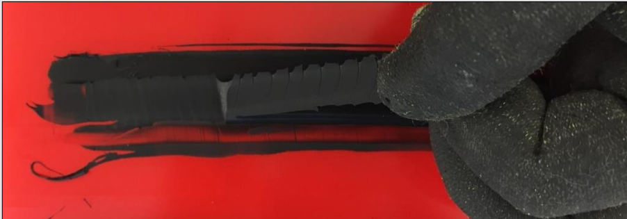
Figure 24: Peel adhesion test: pulling the bead apart, result: 100% cohesive failure
