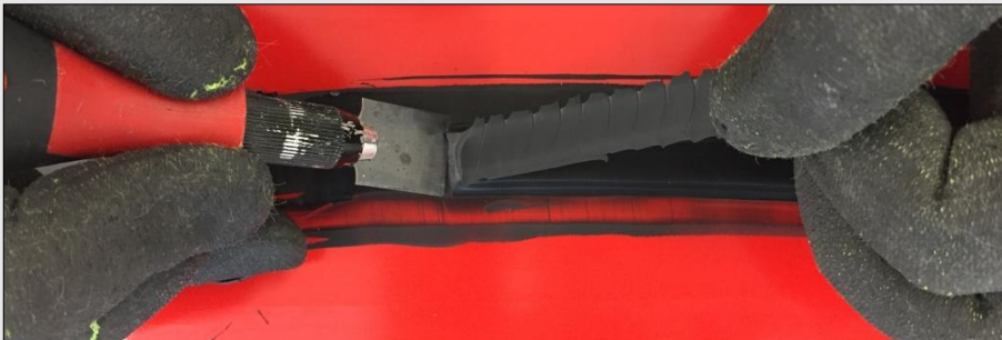
Figure 25: Peel adhesion test on enameled glass: cutting the bead while pulling
