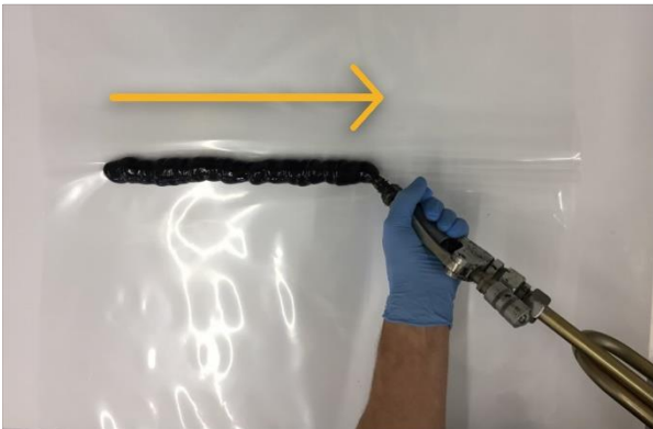
Figure 9: Apply the bead in the fold direction
