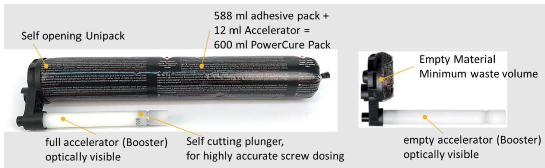
FIGURE 5 PowerCure unipack (Sikasil® WT-66 PowerCure) full and empty – check for usage of accelerator (booster)
