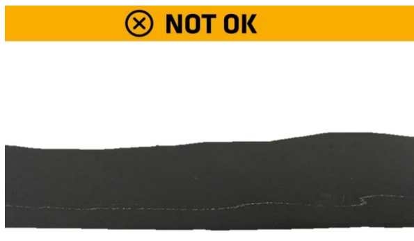
Figure 15: White stripe in material, inhomogeneous mixing
