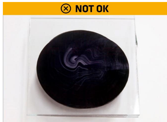
Figure 8: Negative test = inadequate mixing
