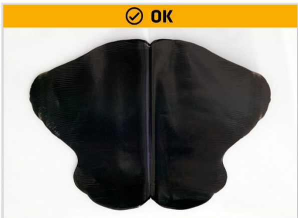
Figure 11: Unfold the foil - Positive test = ideal mixing
