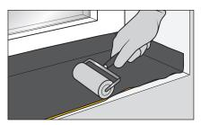
Press the membrane with plastic roller.
