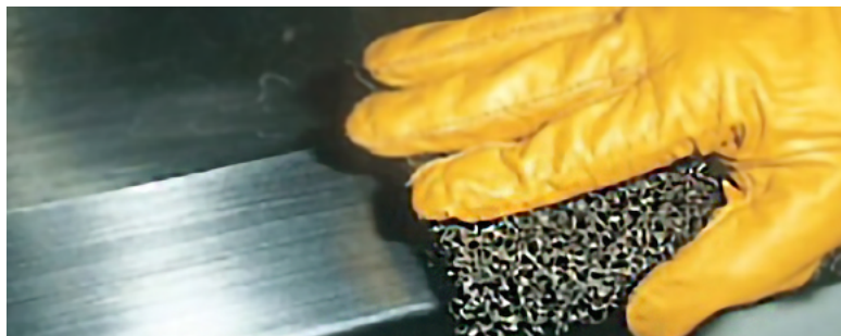
Fig. 6.1 Manual removal of oxidation layer with abrasive pad
