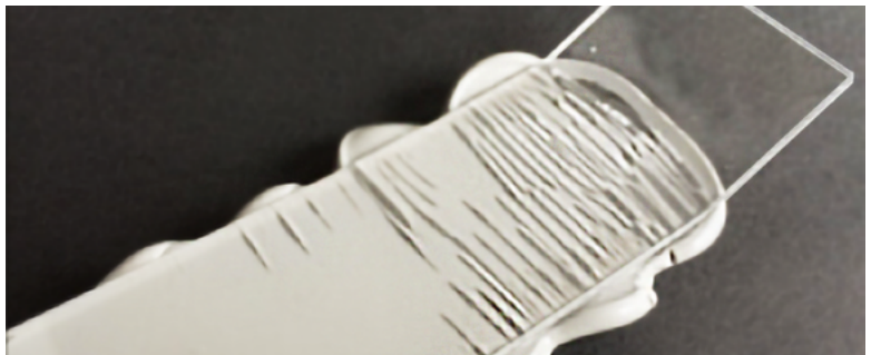
Fig. 10.9 Cracks caused by an unsuitable adhesive
