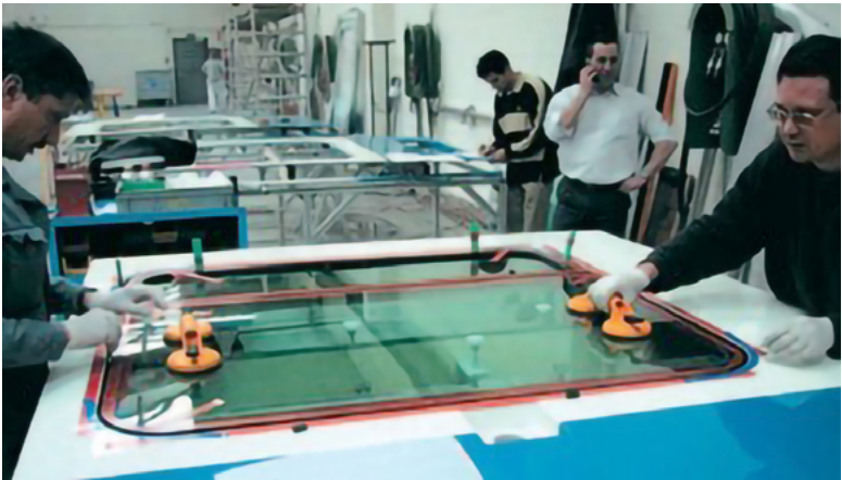
Fig. 7.2 Installation of window glass in sidewall panel
