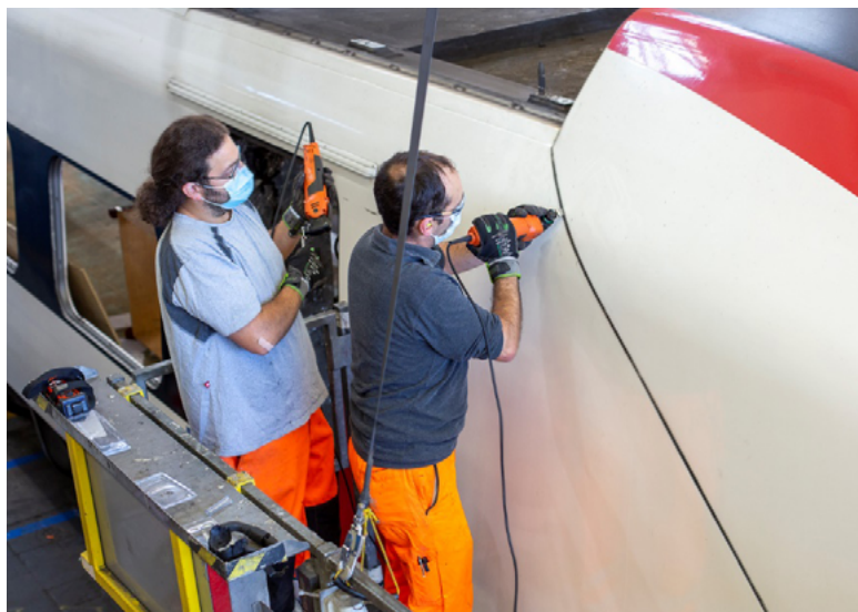
Fig. 10.15 Workers cut the sealant and adhesive with an oscillating knife
