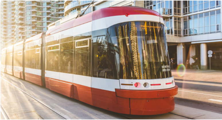
Fig. 1.1 Modern trams owe their stylish looks to a combina- tion of glass, engineered plastics and lightweight metals, bonded together with adhesives
