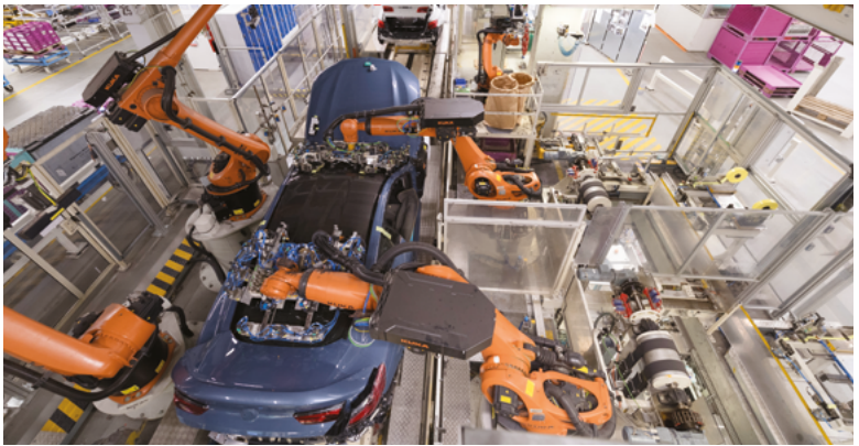
Fig. 8.10 Glazing station of an automotive OEM
