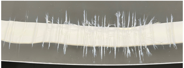
Fig. 10.8 Cracks in transparent thermoplastic material
