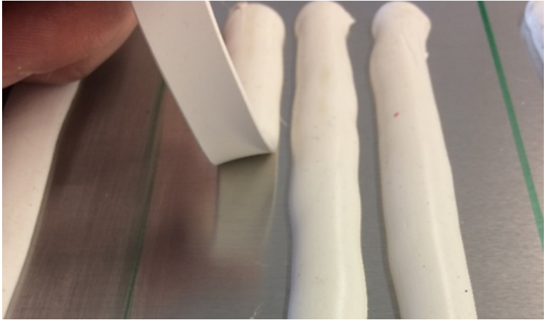
Fig. 9.8 Very poor adhesion with 100 % adhesion loss
