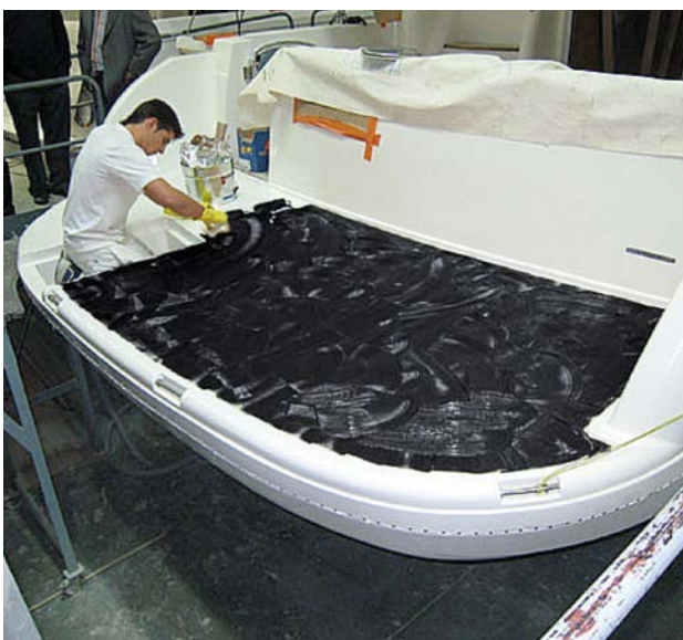
Fig. 26 Application of Sikaflex®-298
