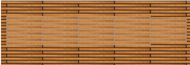
3. Embedded new planks
