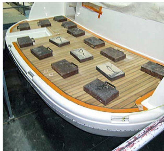
Fig. 27 Holding in place with weights
