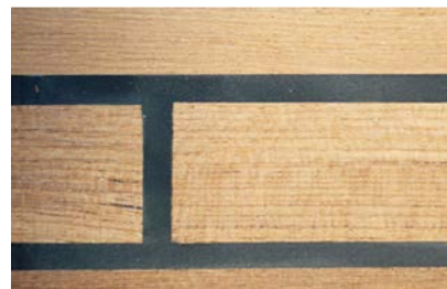
Fig. 29 New teak deck
