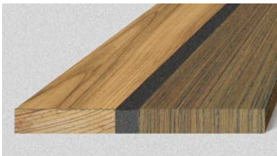
Fig. 1 Left side: laying year rings are not recommended. Right side: standing year rings are best.
