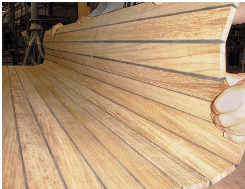
Fig. 23 Deep joint prefabricated teak decking and the strength and flexibility inherent in the adhesive
