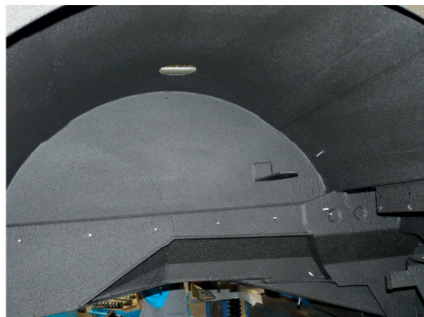
Wheel arch with Sikagard®-6682 applied
