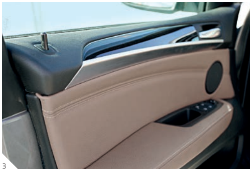
1 Leather wrapped dash board laminated with SikaSense® 2 Center console laminated with SikaTherm® 3 Door insert laminated with SikaMelt®
