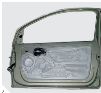
1 Decorative trim parts assembled by using SikaMelt® PUR 2 Water shedder assembly bonding with SikaMelt® PSA
