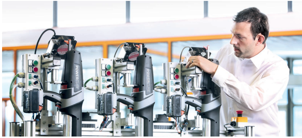
At CEKAtec AG, every PowerCure dispenser is tested in a simulated application before delivery.
