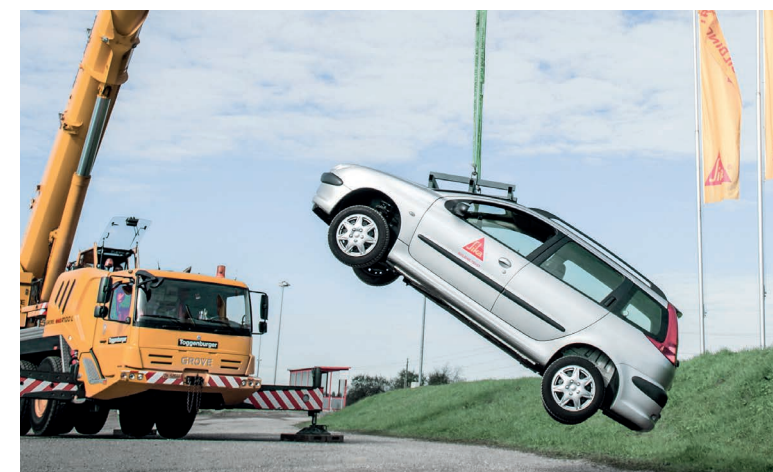
With SikaTack® ELITE, a car can be lifted by its windshield just 60 minutes after installation.
