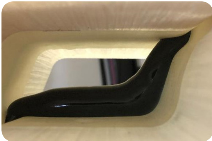
Pumpable baffle in a chassis channel.
