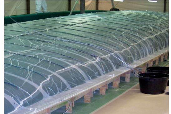
Vacuuminfusion with SikaBiresin® CR131
