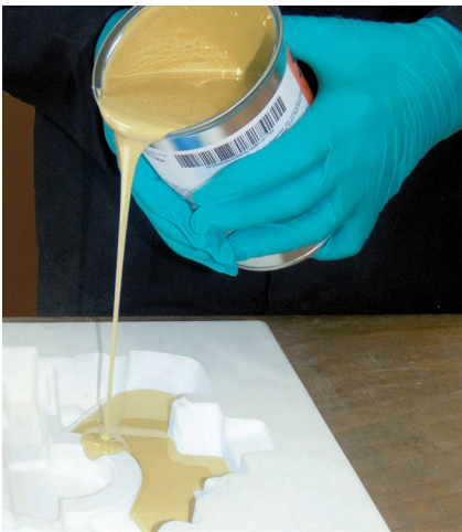
SikaBiresin® F160 with additional fillers for casting of models with thicker sections
