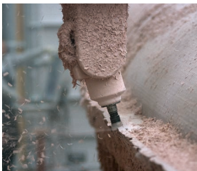
Biresin® M72 paste can be milled easily with low dust formation
