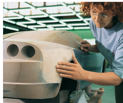
Models milled out of SikaBlock® PROLAB 65 N fulfil highest demands of surface quality
