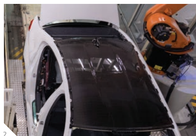
1 1 Crash resistant bonding of mixed material 2 CFRP roof bonding
