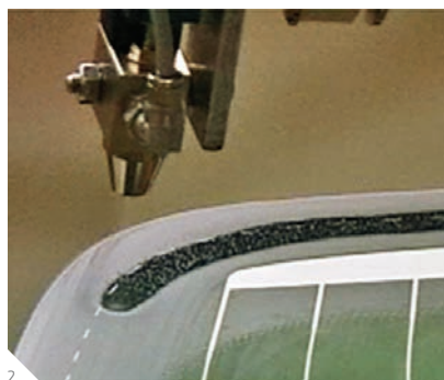
1 "All in one" black primer for glass, ceramic, paints, plastics, SikaPrimer®-217LUM 2 Automated application of water based activator, Sikaflex®-217 LUM
