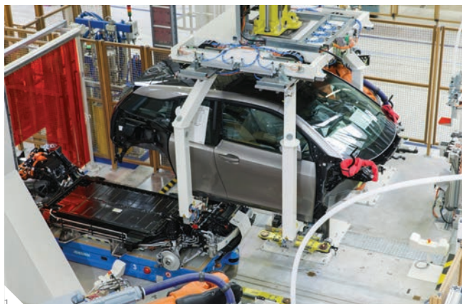
1 1 Crash resistant bonding of mixed material 2 CFRP roof bonding
